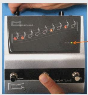
Press and hold Up/Toggle Button while Plugging In the Power
